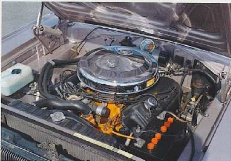
Never say never. This is the OEM air-cleaner top that was delivered with the car, but it has no centered orange 426 Hemi decal on it like most do.
