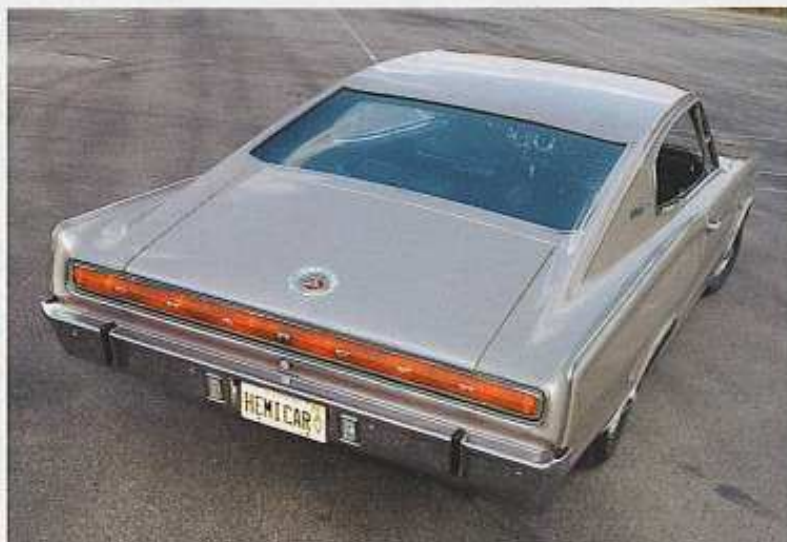
The long red lens across the entire rear states "Charger," and it's fragile; many Chargers from '66-'67 that turn up have this item either damaged or missing.
