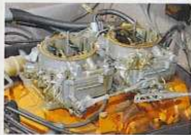
The pair of Carter AFBs the factory selected worked pretty well on the new dual-plane street intake, which was heated with an exhaust-tube system routed up from the passenger-side headpipe. Since Cora never needed to get the engine reworked for racing, these are basically untouched, other than by Keith's very careful cleaning. Details abound.
